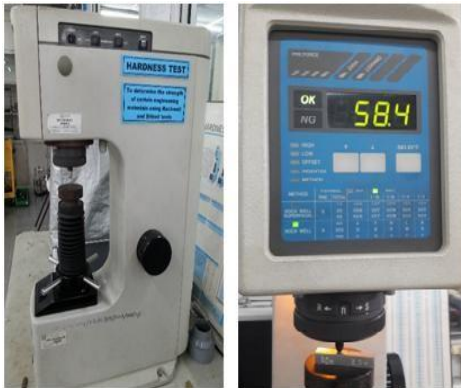
Figure 6. Rockwell hardness test machine and a specimen under the test.
