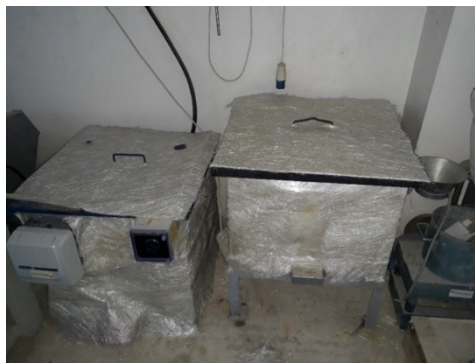
Figure 3. Curing water tanks at 40, and 60°C.
