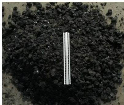
Figure 1. Slag in aggregate form.
