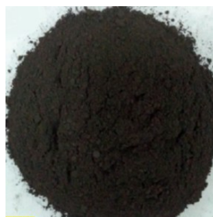
Figure 2. EAFS after grinding.
