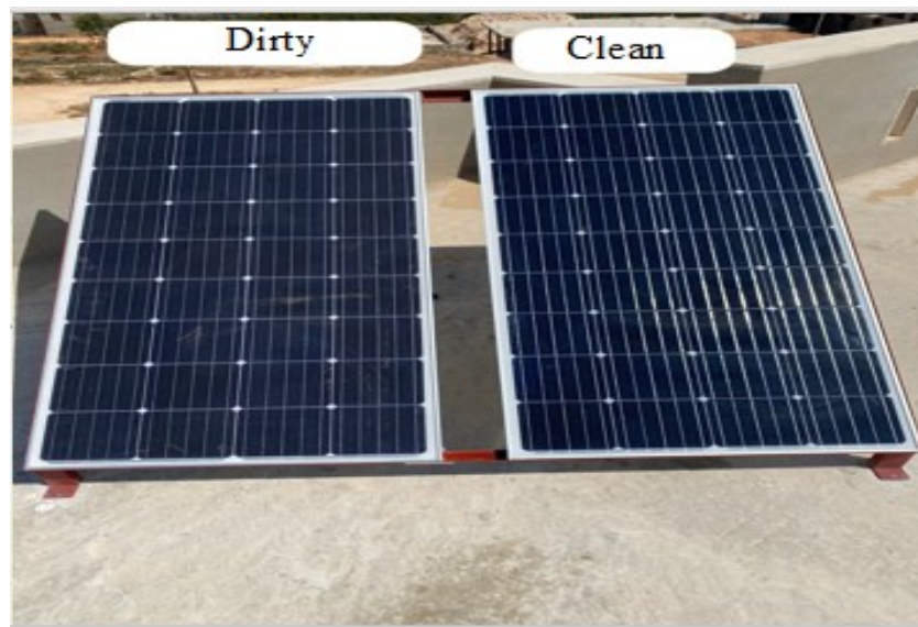
Figure 1. The experimental setup of two identical PV panels
