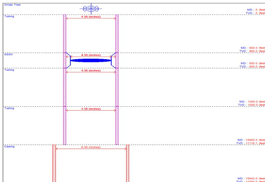
Figure 1. Downhole equipment sketch Before Gas lift
